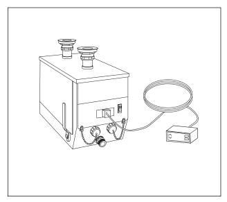
Figure 2. Hydro-Heater with Remote Electronic Controller
